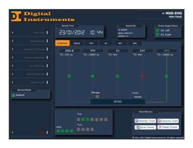
When locked to GPS, MXS-EVO became a cost effective G.811 source for SDH, SONET or PTSN applications. Thanks to high stability OCXO, MXS-EVO is able to provide excellent holdover performance. This equipment is managed by web based GUI, and/or SNMP. For local configuration LCD and keypad can be used. Feature of MXS-EVO is also the possibility to characterize the quality of the sources provided to the equipment through the analisys of the  $\Delta f/f$  ratio of each source.
