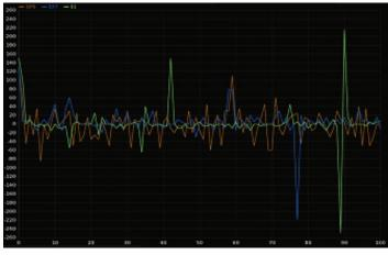
The analysis is supported by a graphical display of  $\Delta f/f$  ratio vs. time. In addition it's possible view the delay (nsec) between PPS generated by internal GPS Receiver and the four different sources, both on web and LCD display.
