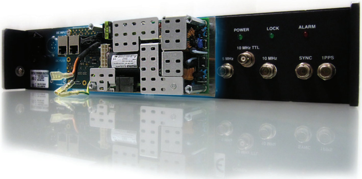
EASY-CS3 mounted on Microsemi CsIII Model 4310B (unboxed view)
