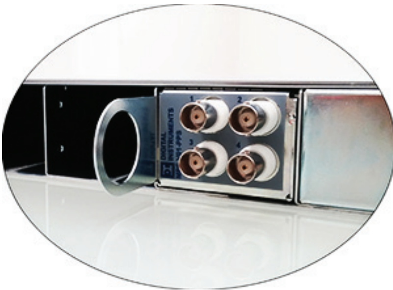
MPE-V01 back panel. The EXP-PPS module is plugged inside and ready to be used.
